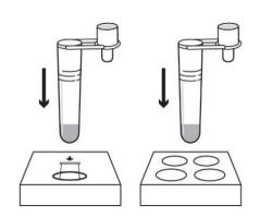
2. Remove the foil from the top of the extraction buffer tube. Place the tube in the tube holder.
