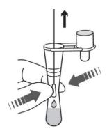
6. Attach the dropper tip firmly onto the tube. Mix thoroughly by swirling or flicking the bottom of the tube.
